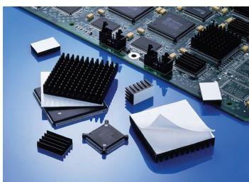
**Thermal Attachment Tapes** are double-sided adhesive tapes which provide a thermal interface between electronic components and heat sinks. This eliminates the need for mechanical attachment such as screws, clips, and rivets. They can be die-cut in various forms and supplied on continuous rolls.
